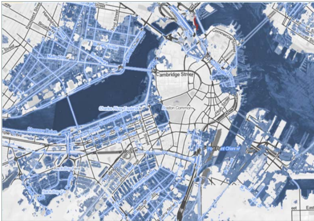
Figure 37. Areas of Boston MA within 5 feet elevation of the 2015 high tide line. Adapted from Climate Central, 2018a. There is an 83% chance of at least one flood of 5 feet or more between 2016 and 2050, and by 2060 the chance is nearly 100% (Climate Central, 2018b). The blue areas affected by a 5-foot flood would be 4 feet under water with a 9 foot flood above the 2015 high tide line as shown below.
